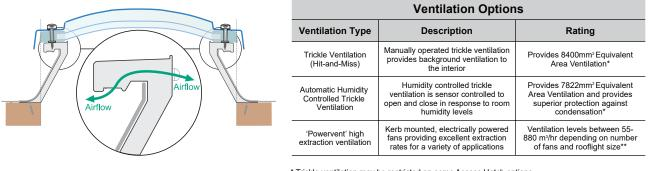
Trickle ventilation may be restricted on some Access Hatch options \*\*1-4 extraction fans available - maximum quantity dependent on rooflight size.
